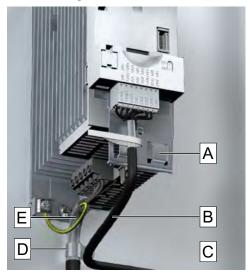
Alternatively, the motor cable can be shielded on an optional motor shield plate.
