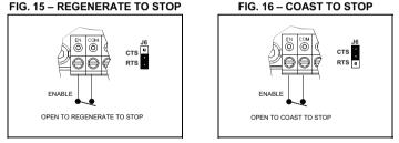
\*FWD Accel and REV Accel do not affect the stopping time when the enable circuit is opened.
