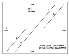
The DB trimpot also determines the amount of delay that will occur before regeneration starts. Regeneration occurs when the applied load torque is in the same direction as the motor rotation.
