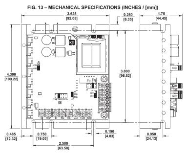
F. Voltage Following – An isolated analog voltage can be used in lieu of main speed potentiometer. Connect signal to terminals "SIG" and "COM." Note: Terminal "COM" is common. A positive signal to terminal "SIG" will produce a positive output to motor. A negative signal to terminal "SIG" will produce a negative output. A 0 to ±10VDC is required to operate control from 0 ± full output. Note: Jumper J4 must be
