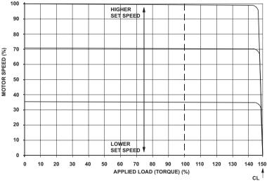
FIG. 7 – TORQUE CONTROL MODE (Linear)
