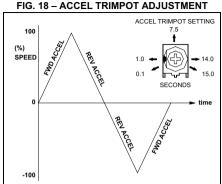
voltage to reach full output in the reverse direction and the time it takes for the control voltage, in the forward direction, to reach zero output. (REV ACCEL is the Forward Decel.)
