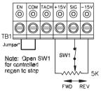
\*Note: A jumper must be wired to EN and COM in order for control to operate.
