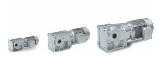
Our efficient bevel gearboxes boast high permissible radial forces, closely stepped ratios and low backlash. They are available in 2-stage and 3-stage designs with a maximum torque of 20,000 Nm and ratios of up to i=360 depending on your individual requirements.
