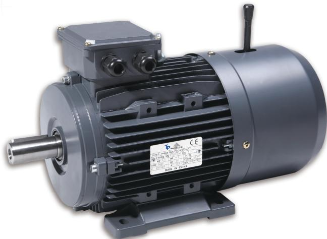
The brake-motors of the MSBCCL series result from coupling an asynchronous three-phase motor and an electromagnetic D.C. brake unit. Due to their reliability and operating safety, as well as their quick braking time (connection & disconnection time = 5~80 milliseconds) they are suitable for a great variety of applications, such as:
