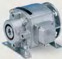
Clutch-brake combinations Drive, hollow shaft, B14 flange – output, hollow shaft
